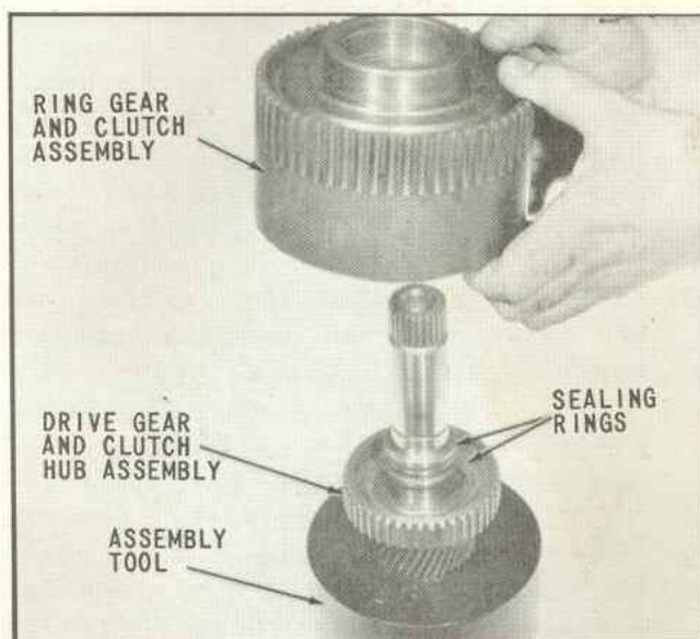
Fig. 47 Assembling Ring Gear and Clutch Assembly on Drive Gear
